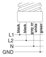
Be sure to install an appropriate conduit box (not furnished) to connect the oven. Don't shorten the conduit to facilitate service! The conduit should be routed to permit the removal of the oven.
